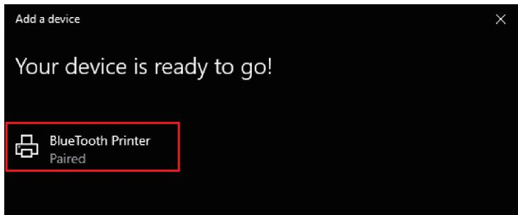
**Step 7:** The Bluetooth printer will be automatically assigned a COM port, pls click “More Bluetooth options” and check the Bluetooth Settings and find out the COM port what the Bluetooth Printer is assigned.
