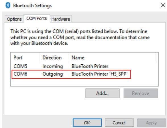
**Step 8:** Open the Printer Driver “Properties”, select the specific COM port which bluetooth printer is used. Remember that the COM port should be setting the corresponding baud rate same as Bluetooth serial port.(Factory Default Baud Rate : 115200, N, 8, 1.).
