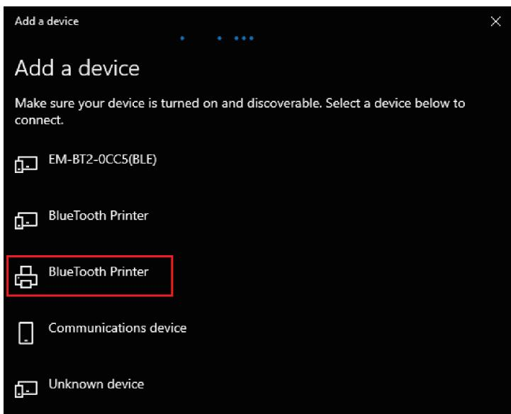
**Step 5:** Enter the PIN(1234) for Bluetooth Printer, then connect:
